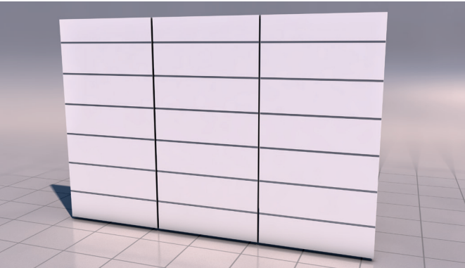
Panel wall light grey Type of construction: Front MDF or particle board, light grey, double varnished. Pilaster-strip aluminium U-profile, anodised. Open side visible, embedded flush with the adjacent areas.
